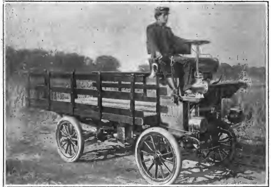
MAXWELL 3,000-POUND TRUCK, DRIVEN BY 18-H.P. OPPOSED CYLINDER MOTOR IN FRONT.
